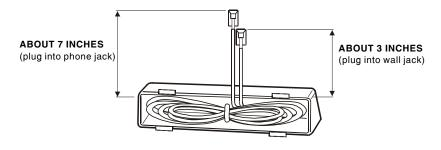
WALL MOUNT ADAPTOR SNAP THIS INTO THE BOTTOM OF THE PHONE AS SHOWN ON THE NEXT PAGE
